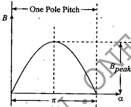
The figure as shown above represents the sinusoidal flux-density distribution in the air-gap of a d.c. machine.
