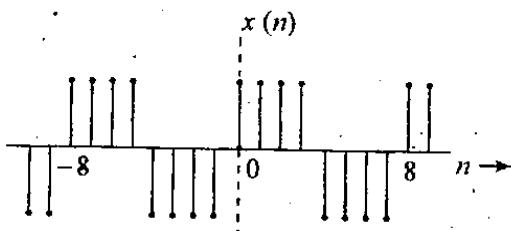
What is the fundamental frequency of the discrete-time square wave, as shown in the above figure ?
