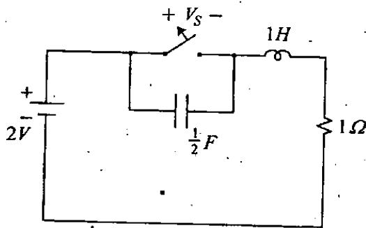
The network shown in the above figure is in steady state with the switch closed. At  $t = 0$  the switch is opened. Which of the following gives the voltage across the switch,  $V_s$  and  $\frac{dv_s}{dt}$  at  $t = 0^+$  respectively?
