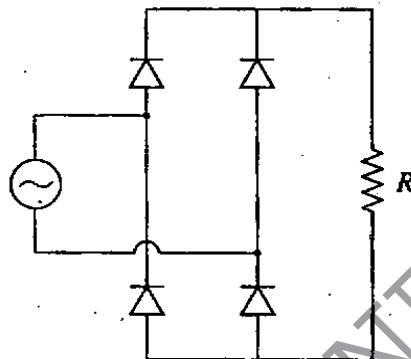
In the single phase diode bridge rectifier as shown in the above figure, the load resistor  $R = 50$  ohms. The source voltage  $V = 200 \sin \omega t$ , where  $\omega = 2\pi \times 50$  radians per second. What is the power dissipated in the load resistor?
