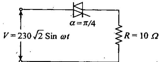
The triac circuit shown in the above figure controls the a.c. output power to the resistive load. What is the peak power dissipation in the load ?
