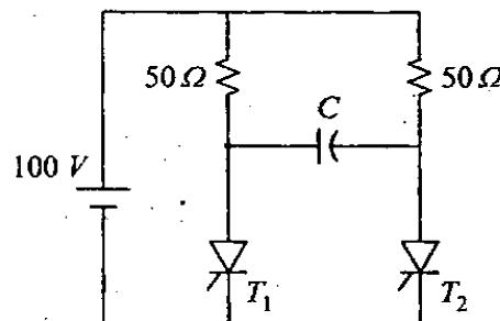
A voltage commutation circuit is shown in the above figure. The turn off time of the SCRs is 50 micro-second. A safety margin of 2 is to be incorporated. What will be the minimum value of capacitor to be provided for proper commutation?
