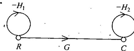
With reference to the signal flow graph shown above, which one of the following will be the overall transfer function ?
