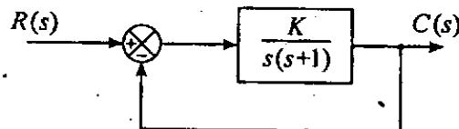
For the system shown in the above figure which one of the following gives the correct range of values of  $K$  so that the steady state error for an input  $r(t) = 0.2t$  is less than 0.004 ?
