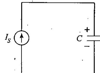
In the circuit shown in the above figure, the initial voltage on the capacitor,  $V(0) = 1$ , before  $I_S$  is connected at  $t = 0$ . If  $C = 2F$  and  $I_S = 2A$  for  $t > 0$ , then what are the values of the voltage (in volts) and charge (in coulomb) on the capacitor at  $t = 3$ .
