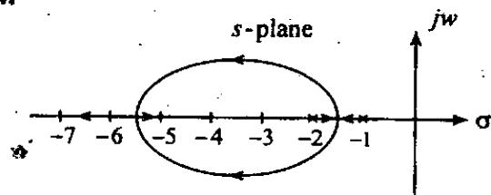
The figure shown above represents root locus of a unity feedback control system. Which one of the following is the correct open loop transfer function of the system ?
