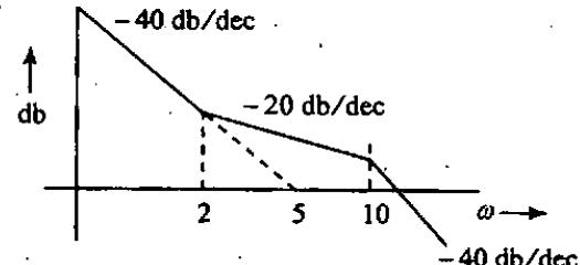
Which one of the following gives the transfer function of the minimum phase system whose Bode plot is shown in the above figure ?
