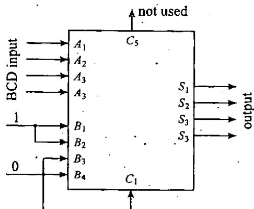
What is the output of the code converter constructed using a 4 bit full-adder MSI circuit as shown in the above figure ?
