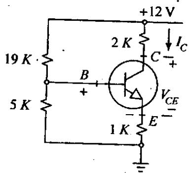
In the circuit shown in the above figure, what are the values of the quiescent collector current ( $I_C$ ) and collector-emitter voltage ( $V_{CE}$ )? (Neglect the effect of base current and assume large  $B$  and  $V_{BE} = 0.5$  V)
