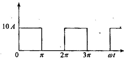
A MOSFET rated for 15 A, carries a periodic current as shown in the above figure. The ON state resistance of the MOSFET is 0.15 ohm. What is the average ON state loss in the MOSFET?
